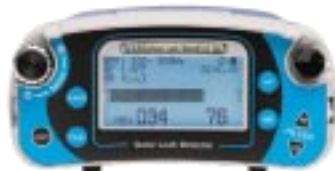
LD-18 Amplifier showing filter settings, bar graph and numeric display of sound loudness, and minimum sound level detected
