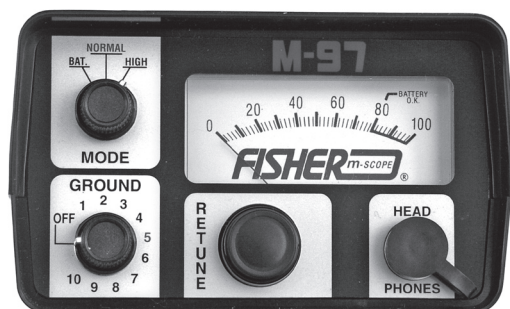
M-97 Control Panel
