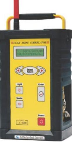
High sensitivity, small diameter LC-2500 Sensors standard for metal pipes and A/C mains.
